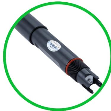
NBL-S-TH/The soil temperature and humidity sensor has stable performance and high sensitivity, and can measure soil temperature and soil moisture at the same time; by measuring the dielectric constant of soil, it can directly and stably reflect the real water content of various soils. The soil moisture sensor can measure the volume percentage of soil moisture and is a soil moisture measurement method in line with current international standards.
